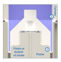
The diaphragm ends are fixed to the piston (1) and internal cylinder (2). As the piston moves, the end of the diaphram connected to it moves and the end connected to the cylinder remains stationary. The center of the diaphragm rolls, forcing liquid in/out.
